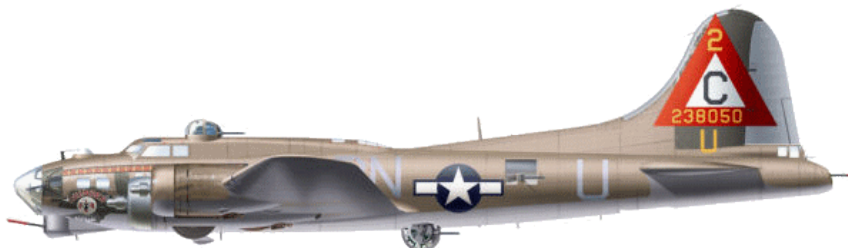
B-17G - OLIVE DRAB AIRCRAFT - RED TRIANGLE "C" TAIL INSIGNIA GRAY FUSELAGE LETTERING - YELLOW LETTERING ON TAIL NOTICE THE B-17G HAS A "CHIN" TURRENT
